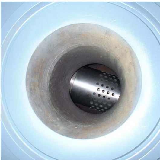
Figure 4: Retainer through side inlet of body
