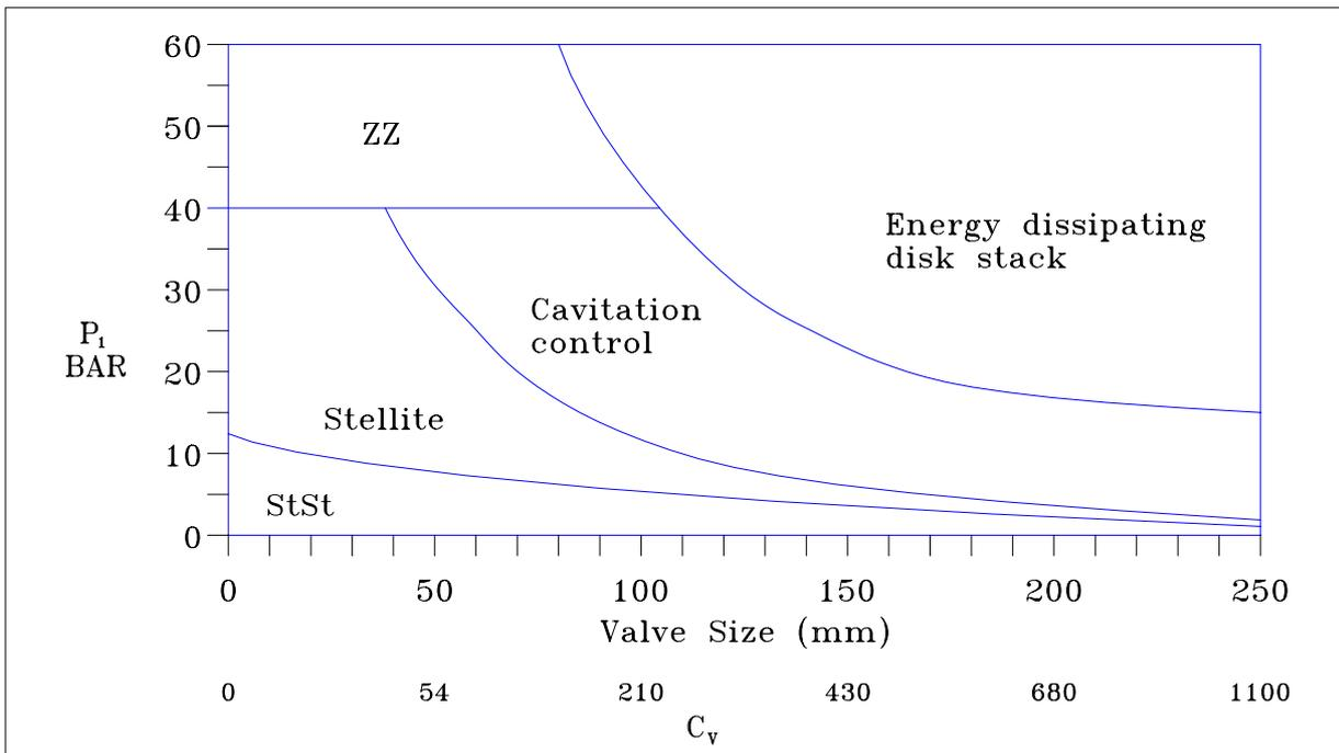
**Figure2:** Trim Selection Guide : Liquid Applications
