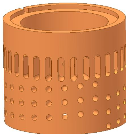
Figure 6: Cavitation control with slots and holes
