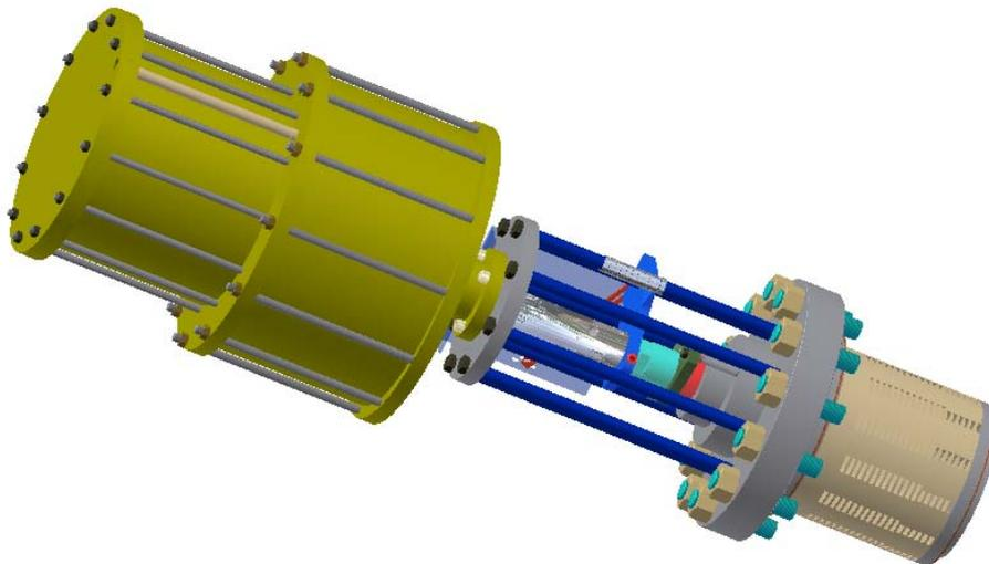
**Figure 10:** Mitech Actuator and Energy Dissipating Disk stack to be fitted to existing body
