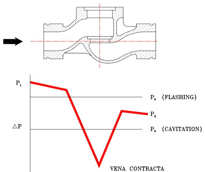
Figure 1: Flow through a control valve
